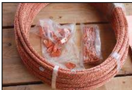
One hundred feet of copper wire, clips, and nails.
